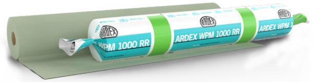
ARDEX WPM 1000 RR is a high-performance, single-ply waterproofing membrane designed for use in areas susceptible to root damage. The membrane contains a premium root inhibitor that repels root growth without killing the root. It is designed primarily for areas covered with, or exposed to soil and plants. Once installed, ARDEX WPM 1000 RR will remain a permanently flexible waterproof lining and bond to most building surfaces.
