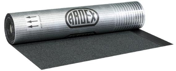
ARDEX WPM 196 is a high-performance, polymer-modified Styrene-Butadine-Styrene (SBS) bituminous tanking membrane with a mineral chip finish. ARDEX WPM 196 has excellent strength and dimensional stability that provides superior waterproofing ability for tanking and below-ground application. ARDEX WPM 196 has excellent cold flexibility and can be applied at temperatures down to -20°C.
