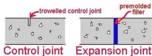
*Control Joint versus Expansion Joint*
