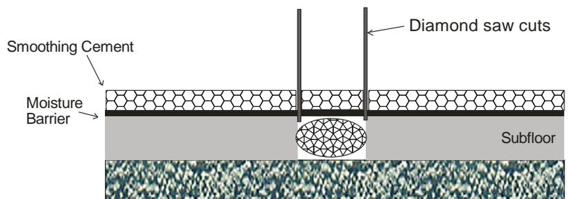
As per step 32 the material from the saw cut has been removed.
