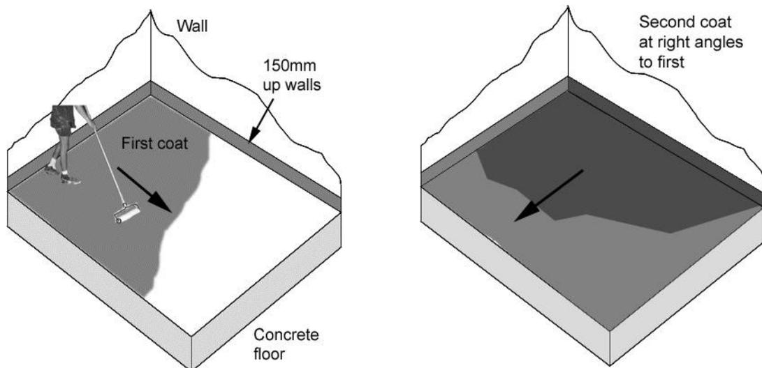
The coats are applied at 90 degree angles to obtain a complete coverage.
