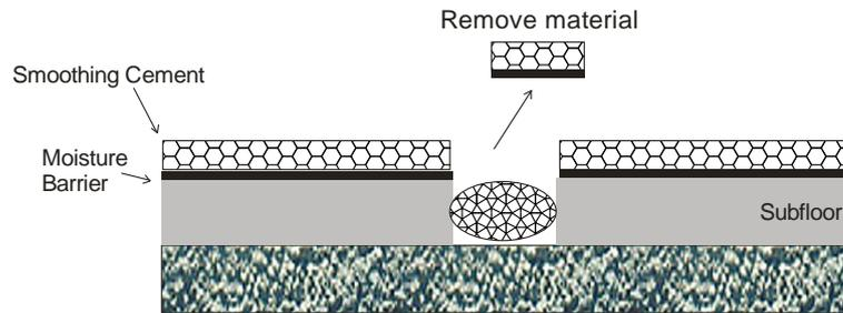
As per step 33 Moisture Barrier is painted thoroughly down into the joint. A suitable flexible sealant system is then installed (may include mouldings or metal extrusions)
