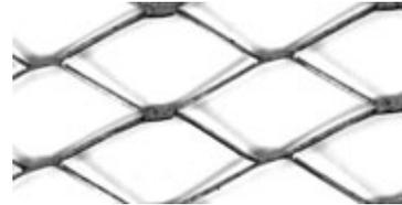
An example of E-glass\* fibreglass matting with 10mm apertures and 2 x 0.75mm thick fibres.
