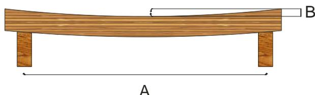
The diagram shows a typical floor or step-tread with the bearer span shown as A and the deflection as B.
