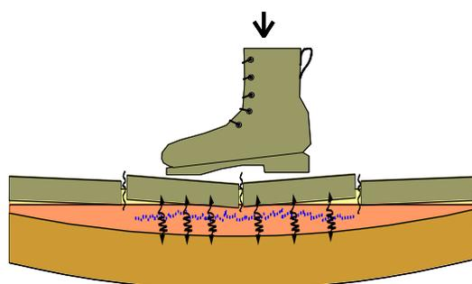
Where the deflection exceeds the recommended limits, or the maximum permissible movement for the adhesive, the adhesive can shear which will result in de-bonded tiles and cracked and popping grout.
