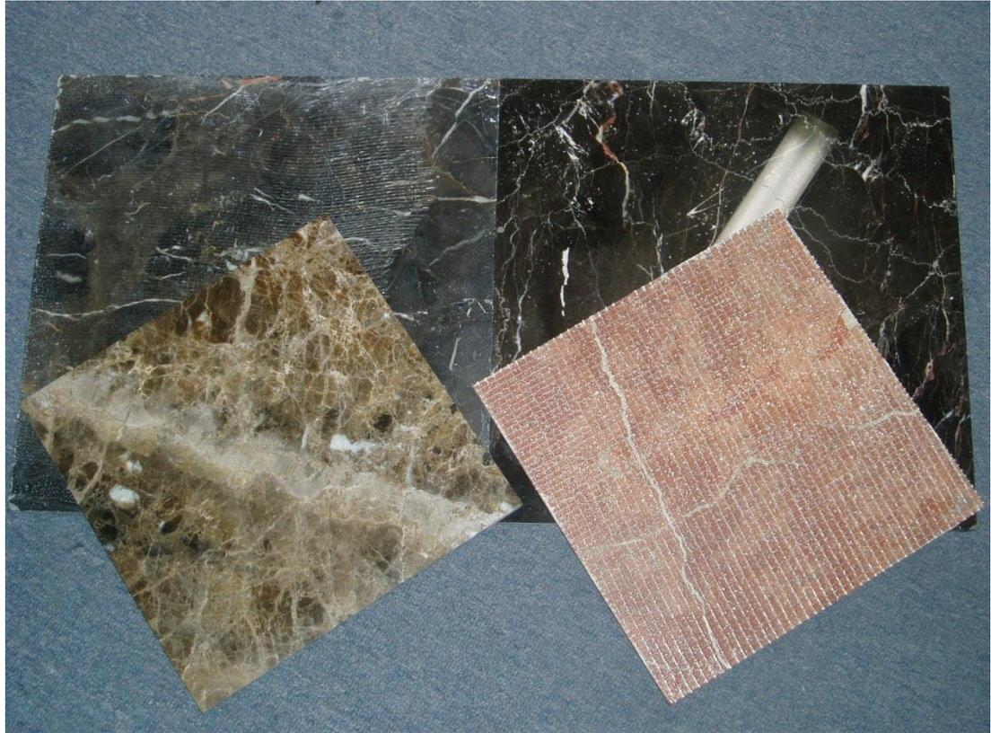
The above examples show how greatly fractured and cracked stone (lower left and upper right shows the polished faces) may be held together by the resin reinforcement backing. In addition, incomplete mesh coverage (upper left) is shown although the resin coating was to all edges of the tile, and the sand particles embedded in the resin (lower right) for better mechanical adhesion to the fixative.
