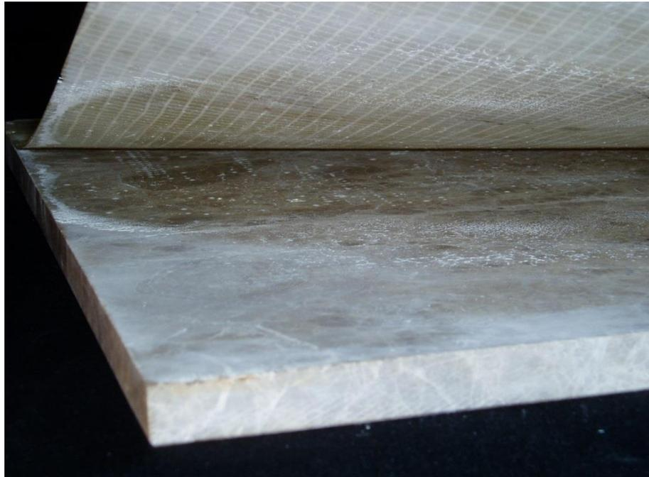
The upper picture here shows the resin backing de-bonding from the stone when unpacked at site.
