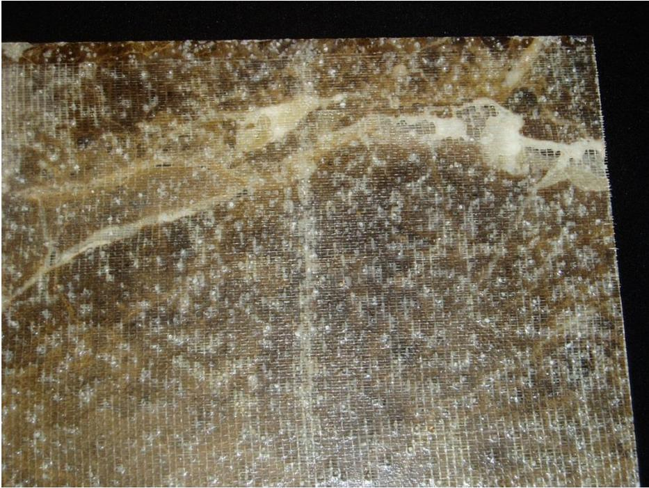
The upper picture shows the sanded resin coating on the back of the tile and also the white vein in the top right with holes all the way through to the front.
