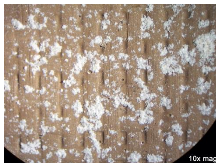
Bare mesh backed tile where rear face of the mesh has been protected a primer coat (WPM368) and then bonded with X77 to concrete. The sample was immersed for several months in water. Coating has protected surface.
